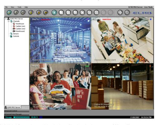
2. Hold the left mouse button and drag the chosen video channel to the new screen division position.
