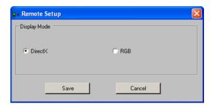
Select the desired Display Mode between **DirectX** and **RGB**. DirectX is the preferred and recommended display mode as it offers substantially higher quality video image. In cases, when DirectX is not installed on the system or is not available (is used by another program), select RGB display mode.
