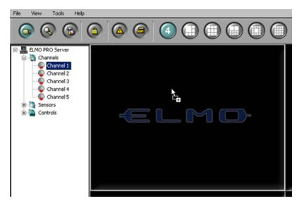
5. Release the mouse button. The chosen video channel will be displayed in the selected main screen division position.
