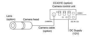
• When connecting or disconnecting the camera cables (for the camera head and camera control unit), always turn off the power switch of the camera control unit first. If not, the camera head may be damaged.
