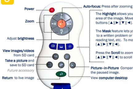
The **Highlight** allows you to emphasize a specific area of the image. Move the highlight using arrow buttons  $[\blacktriangle][\blacktriangleright][\blacktriangledown][\blacktriangleleft]$ .
