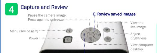
of worksheets, student work, etc. and save them on the SD card. Quickly and easily review later during class by pressing the SD button.
